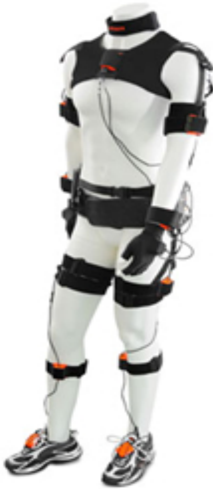
Figure 1.1, An inertial based motion capture system with attached sensors on body [34]
