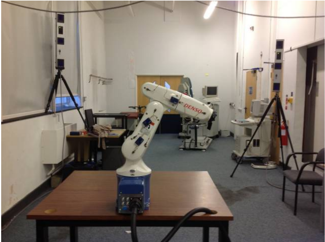
Figure 5.9, Placement of markers which are attached to drive boxes positioned toward or on the mid-section of each rigid body.
