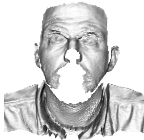
Figure 8: Failure mode: Example scan showing missing nose region which causes failure of the region based approaches due to incorrect PDM fitting and region localisation.
