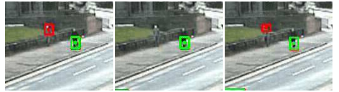
Fig. 9. Example of inconsistent detections interpreted by a PHD filter as clutter and therefore removed. Simple heuristics cannot differentiate these data from real clutter (red: observations; green: output of the PHD filter).
