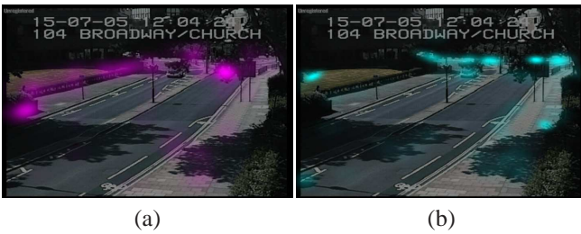
Fig. 8. Learned intensities for scenario S101 from the CLEAR-2007 dataset superimposed on the original images. (a) Birth intensity (note that the major modes are associated with entry areas). (b) Clutter intensities (note that waving vegetation produces clutter that is correctly modeled by the GMM).
