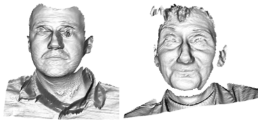
Fig. 3. Sample scans from the GavabDB database showing varying amounts of noise, holes (missing data) and the presence of non-facial regions
