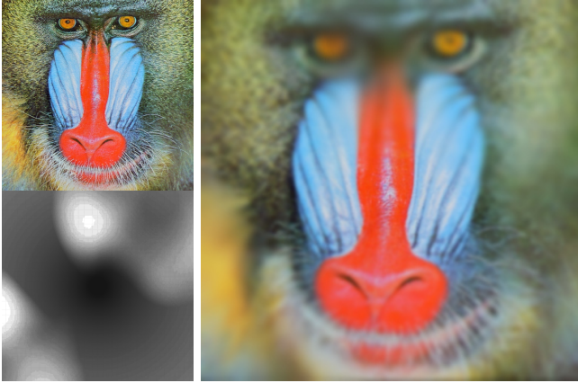
Fig. 6. Top left: raw image ( Mandrill ). Bottom left: blur map based on the visual field of a glaucoma patient [20]; white = maximum ( \sigma = 10 ); black = zero. Right: space-variant Gaussian-blurred image according to the blur map, using the proposed algorithm with N = 8 .
