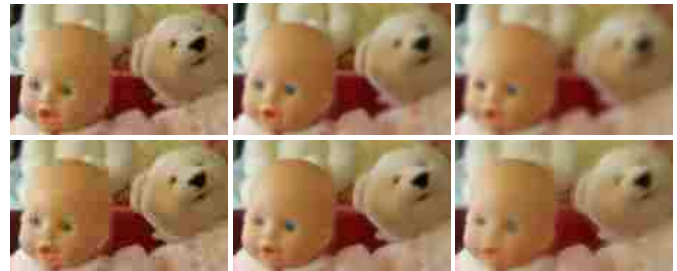
Fig. 16. Zoomed-in portions of Dolls , with foveation preblurring (top) and depth-based preblurring (bottom), with (left to right) blur levels 3, 5 and 10 and JPEG bitrates 0.4 bpp, 0.5 bpp and 0.4 bpp.
