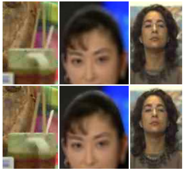
Fig. 15. Zoomed-in portions of sample test images of (left to right) Cones (blur 5, 0.4 bpp), Akiyo (blur 10, 0.4 bpp) and Silent (blur 5, 0.4 bpp). Top row: foveation preblurring; bottom row: depth-based preblurring. All these images yielded statistically significant results in at least one of the two test types, all in favour of depth-based blurring.
