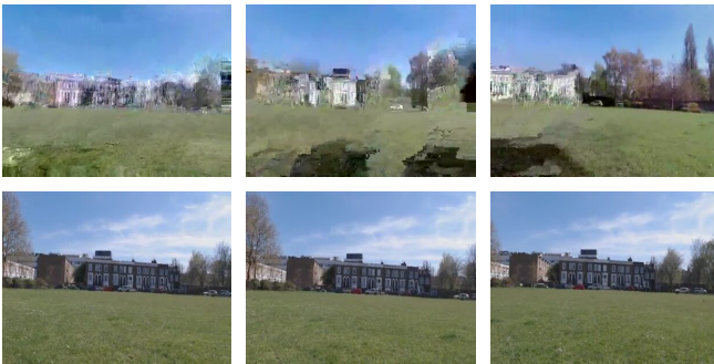
Figure 4: Sample frames representing received video quality with CBR 6 Mbit/s encoded at 128 kbit/s (top row) and our rate adaptive scheme (bottom row) for a multicast video stream.
