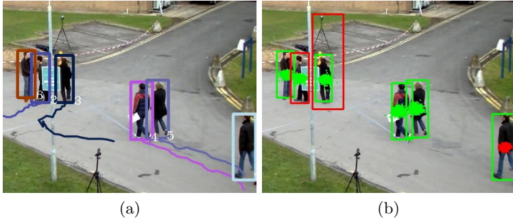
Fig. 4: Example of newborn particles generated at frame 43 (crop) in PETS09-S2L1. (a) Color-coded target identities; (b) existing particles (green dots) and newborn particles (red dots). The newborn particles initialize a new trajectory from an un-associated strong detection.
