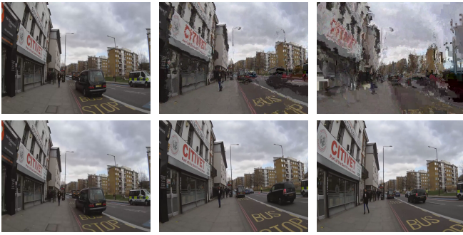
Fig. 6. Three sample frames captured at 2 s intervals representing received video quality with CBR 6 Mbps (first row) and rate adaptive scheme (second row) for a multistream video multicast.
