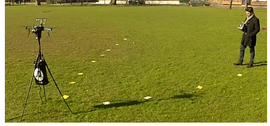
Fig. 4. Experimental setup. A loudspeaker is carried by a person who walks in front of the drone that is placed on a tripod. The noiseless sector is indicated with yellow marks on the ground.
