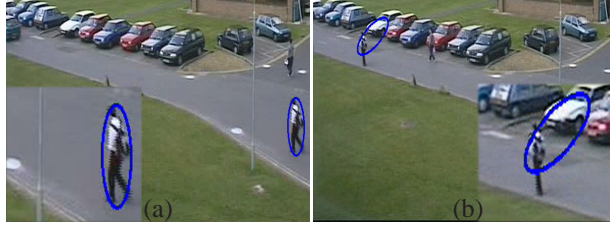
Figure 2: Example of wrong track using colour histograms.
