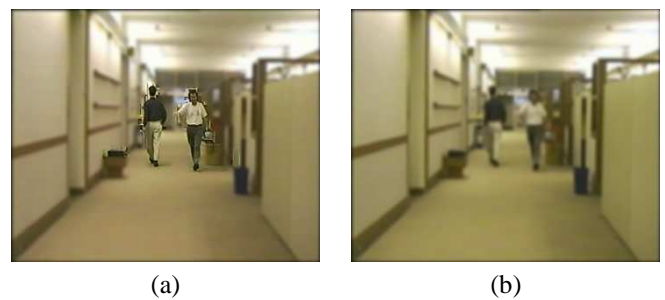
Fig. 4. (a) Selective lowpass-filtering simplifies the information in the background, while still retaining essential contextual information; (b) filtering the entire image inhibits the main content message
